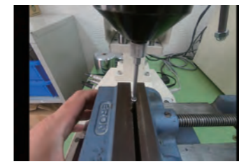
310Slim® breaking torque tested by torque analyzer.
